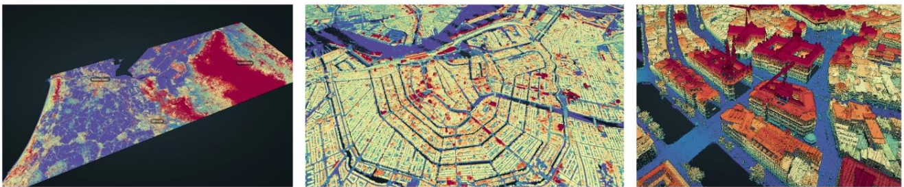
Fig.1 – Illustration of a massive point cloud at three scales with, from left to right, the city of Amsterdam and its surroundings, the downtown and a few building blocks. Image from [6].
