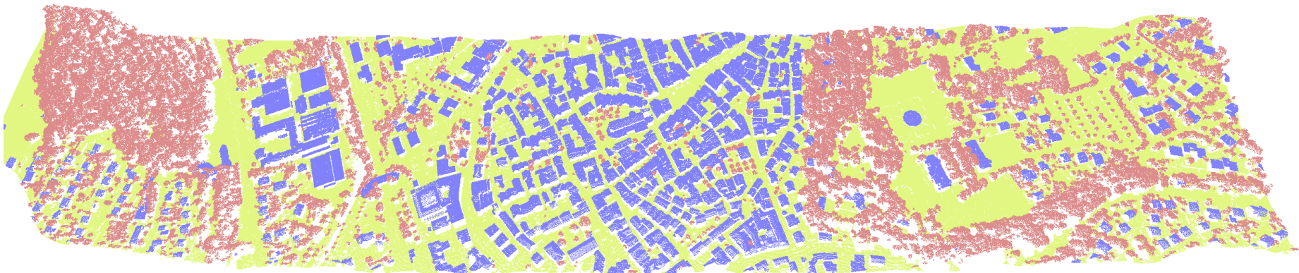
Classified point cloud [color code: blue=building, red=vegetation, yellow=ground, white=clutter]
