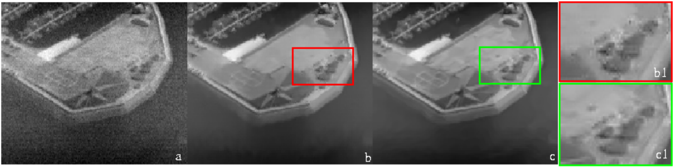
Fig. 7. Infra-red sequence. (a) one image of the original sequence, (b) the corresponding image of the denoised sequence with the non-local filter applied with a patch of size 5 \times 5 and the bandwidth equal to four times the noise standard deviation, (c) denoised image with the proposed motion compensated filter, (b1) Cropped region of (b), (c1) Cropped region of (c).
