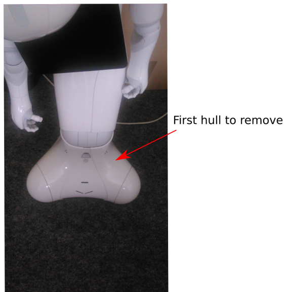
Figure 1: The first hull to remove.
