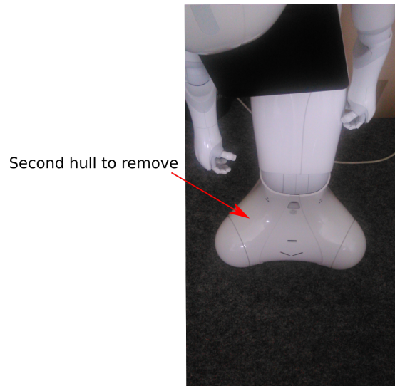
Figure 5: The second hull to remove.
