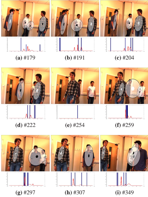
Figure 3: Results obtained with the CTMS3 sequence from the CAVA data set: Time intervals #179, . . . #349. The ellipses correspond to the 3D covariance matrices projected onto the image. The circle at each ellipse center illustrates the auditory activity: speaker emitting a sound (white) or being silent (black) during each time interval. The plot associated with each image shows the auditory observations as well as the fitted 1D mixture model.
