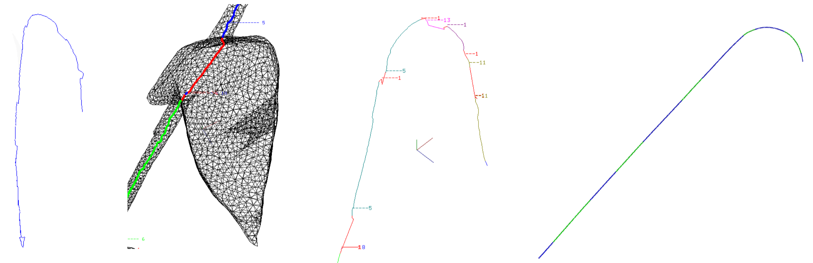
Embedded Reeb graph is noisy (left) because of poor approximation in leaflet areas (centre left). Segmentation (centre right) and spline-based filling generate a smoother curve (right).
