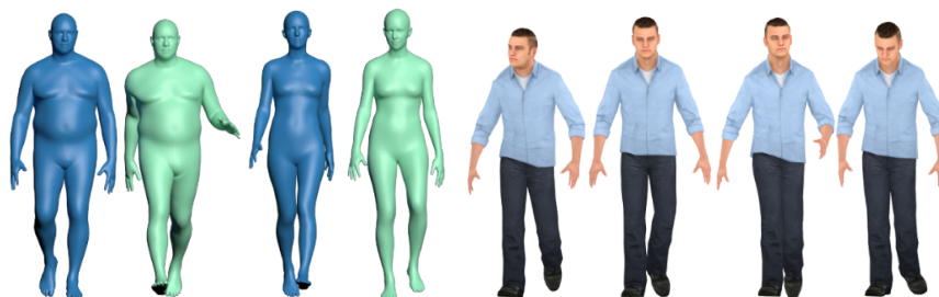
Figure 1. In this project, we want to automatically personalise motions to account for inter-individual variations. Left – Examples of variations due to morphology: appropriate (blue) and inappropriate (green) motions for morphology (errors appear around legs and arms, but also in terms of speed, inertia, balance, etc.). Right – Examples of emotional variations depicting angry motions from four actors. Such examples can be captured, but are difficult to synthesise.
