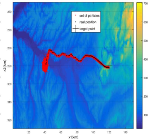
(b) Trajectory from active controller avoiding a flat area
