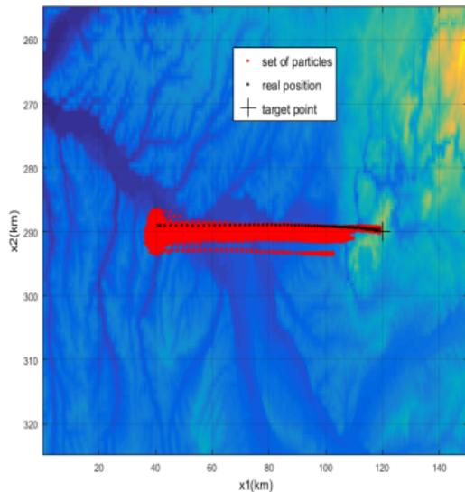
(a) Trajectory from a passive controller over a flat area
