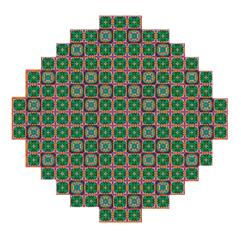
Assemblies are reordered to obtain the most homogeneous neutron flux in the reactor core.
