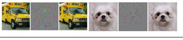
Examples of adversarial images from [4] generated for a given DNN (here AlexNet). (Left) is a correctly predicted sample, (center) difference between correct image and image predicted incorrectly (right) as an"ostrich" (in both cases)
