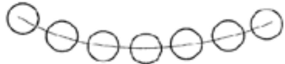
FIGURE 4b. Stroboscopic occurs in a faster action when the object's positions do not overlap and the eye perceives separate images.
