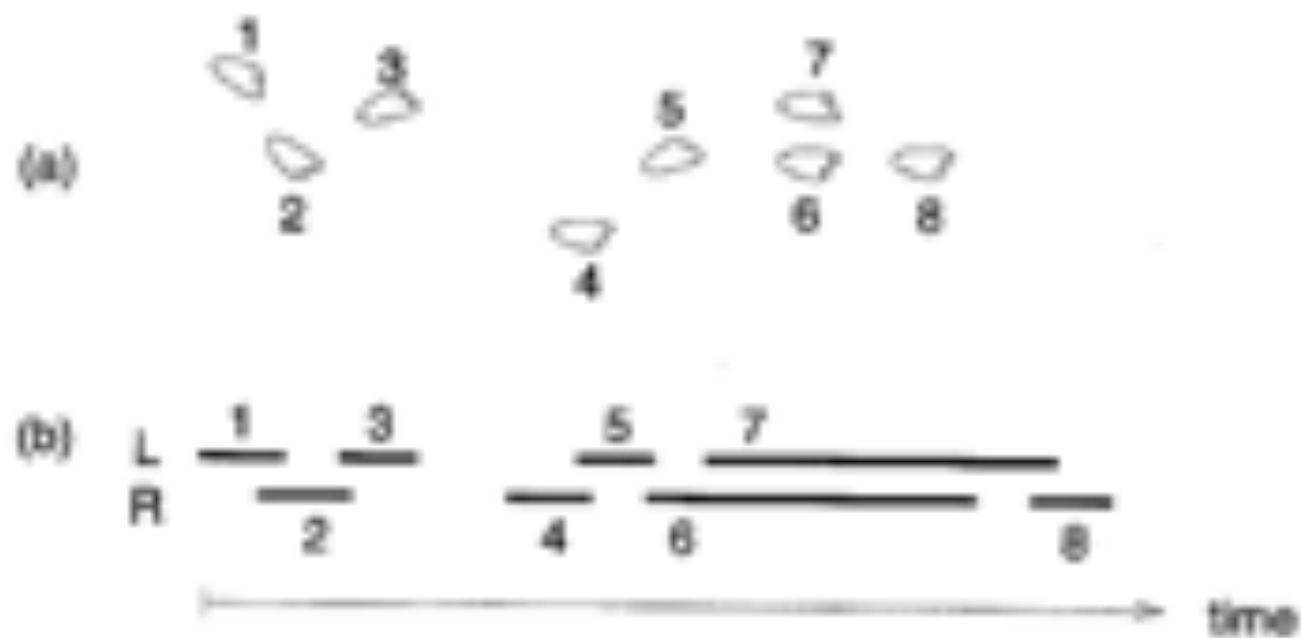
Figure 1: Specification of a Walking Motion (a) plan view of footprints (b) timing diagram.
