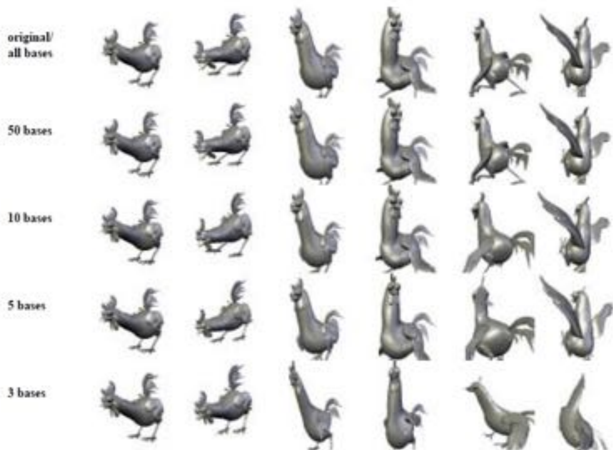
Figure 3: Principal Component Analysis applied to the chicken animation. Prior to the SVD, base shapes are normalized. The sequences above show frames 0, 80, 160, 240, 320, and 400 using different number of bases in the reconstruction.
