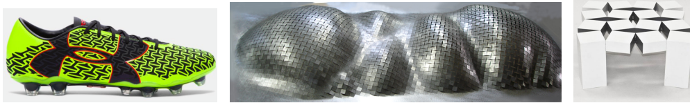
Figure 1: auxetic fabric (UnderArmor sportswear), xSurface in steel from H. Lavani, table from T. Cecil
