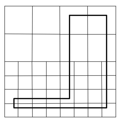
1b / Octree conforming using polyhedral cutting:
