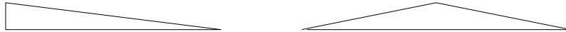
Figure 6: Poorly-shaped element due to quadrant-model interactions, a needle (left) and a flat element (right).
