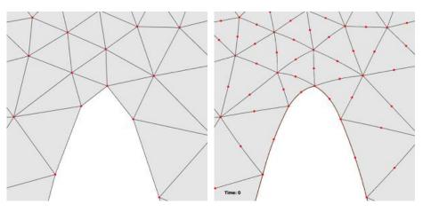
Illustration of a  $\mathbb{P}_2$  curved mesh with the initial mesh in 3D.
