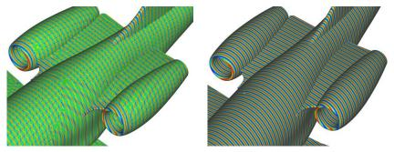
• Example of 2 different solutions rendering on a Dassault Falcon  $\mathbb{P}_1$  mesh with  $\mathbb{P}_1$  and  $\mathbb{P}_3$  solution.
