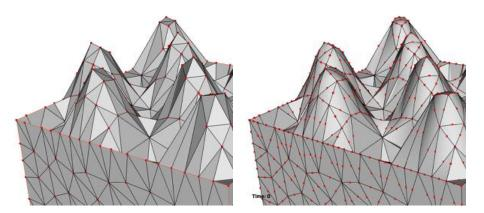
Illustration of a  $\mathbb{P}_2$  curved mesh with the initial mesh in a more complex case of a high-lift 3D. Surface and volume mesh.
