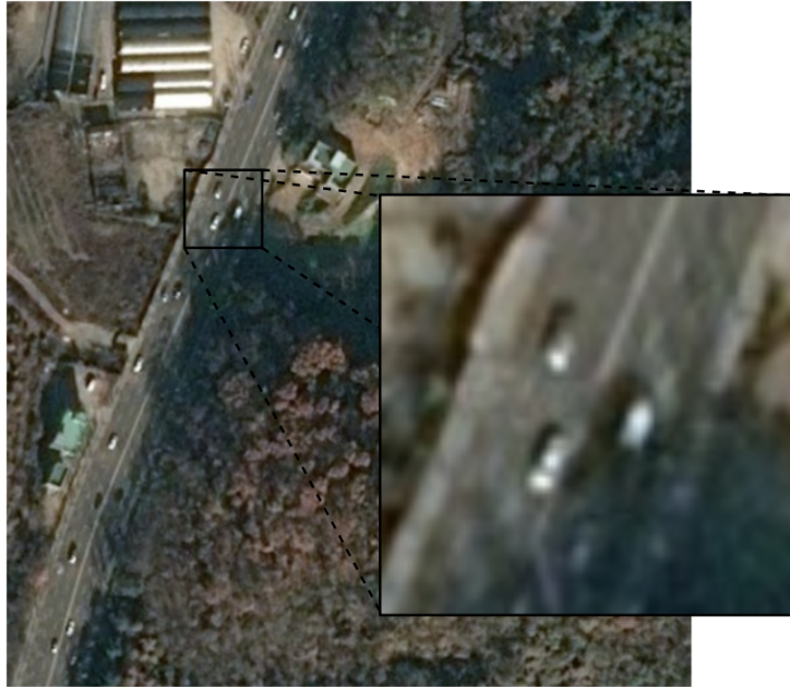
Figure 10: From that sample of data we can observe the inconsistent contrast of vehicles on the road along with drastic illumination changes and the small size of target objects (only a few pixels wide) that make the detection not straightforward
