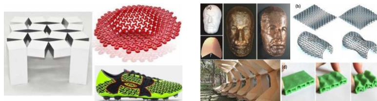
Figure 1: Examples of metamaterials: their mechanical behavior is governed by their geometric structure and not by the material they are fabricated of.
