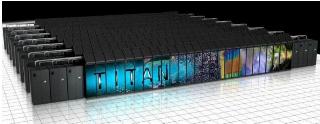
Oak-ridge Titan supercomputer. 200 cabinets, 18 688 nodes, AMD 16-cores + NVIDIA TESLA, 20+ Pflops
