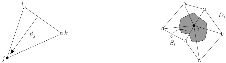
Figure 2: Nodal normals (left), and median dual cell S_i and nodal stencil \mathcal{D}_i (right)
